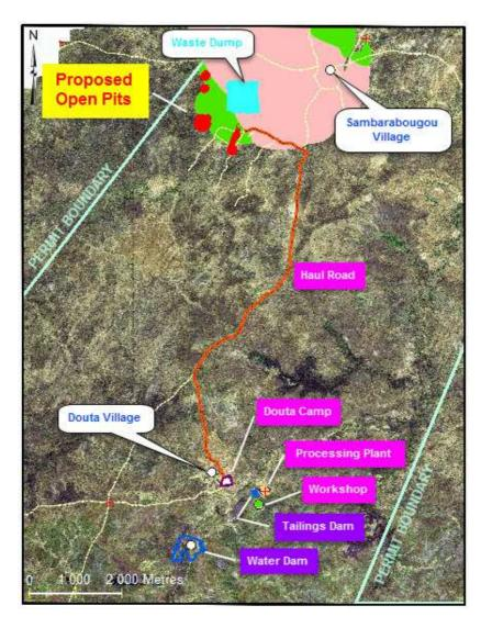
Figure 4 – Project Layout – Mine and Processing Plant
