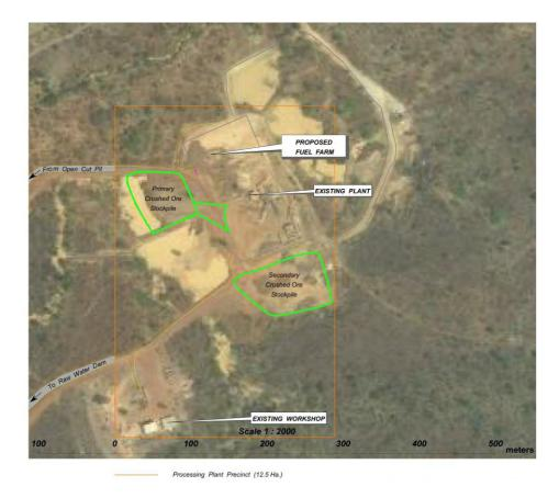
Figure 2 – Processing Plant Footprint
