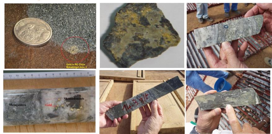
Gold mineralised structures associated with silica –carbonate-sericite –pyrite-arsenopyrite and pyrrhotite.
