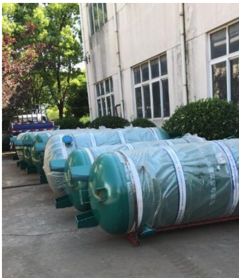
Compressed air receivers
