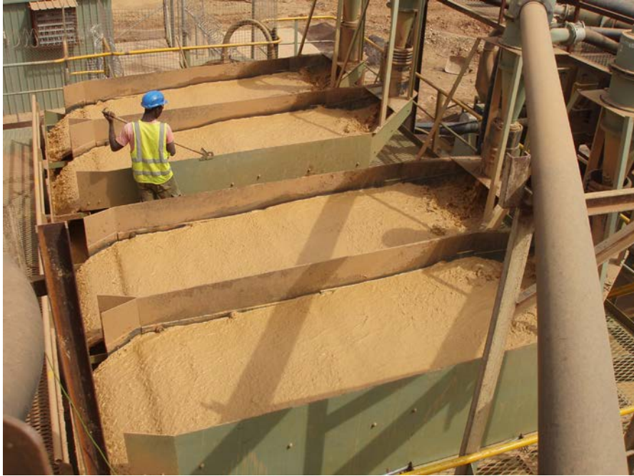
Figure 7 – Four gravity jigs in operation
