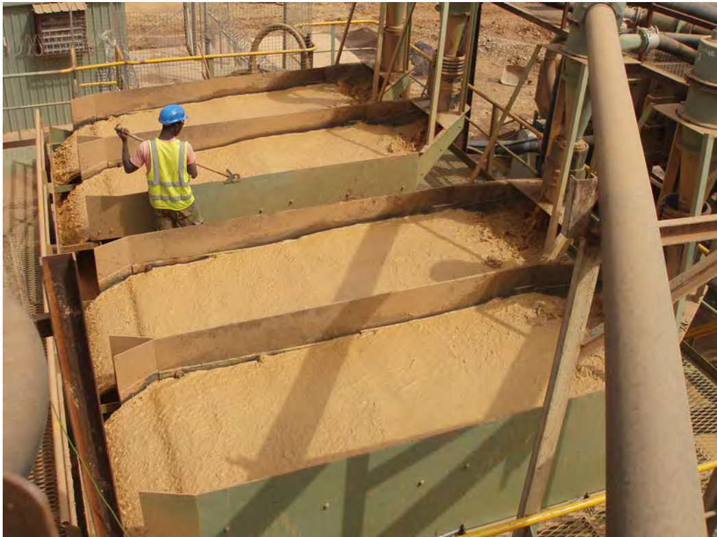
Figure 9 – Four existing gravity jigs in operation
