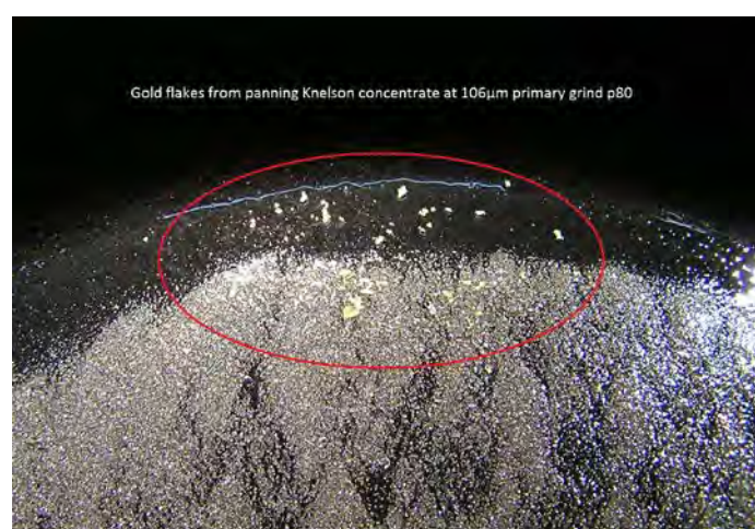
Figure 6 - Gold Flakes in Pan Concentrate for 106 micron Primary Grind
